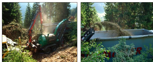
Chipping of slash directly into the transport vehicle; in the left picture the slash concen
