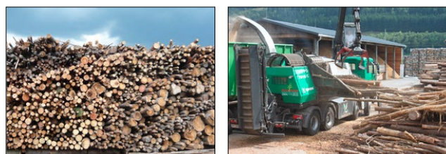
Roundwood is chipped after the right kind and duration of storage © WV Stmk
