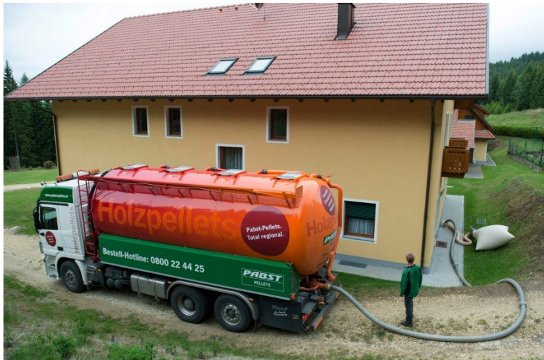
Unloading of pellets at the customer © Pabst GmbH
