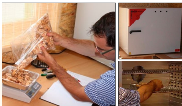
drying of a chip sample in a drying cabinet (Wittkopf 2004).
