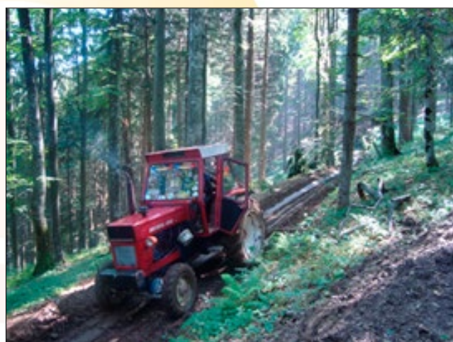
Fig. 3. Low investments for own timber harvesting – a farm tractor adapted for forest operations
