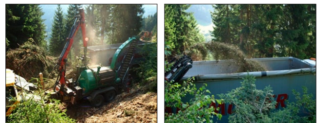
Chipping of slash directly into the transport vehicle; in the left picture the slash concen
